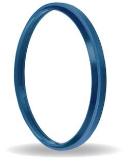
Merkel Wiper PU6 / PH6 is a single-acting wiper made of polyurethane or Hytrel with supportive segments to avoid twisting, a slightly rounded wiper lip and a static sealing edge at the outside diameter.
