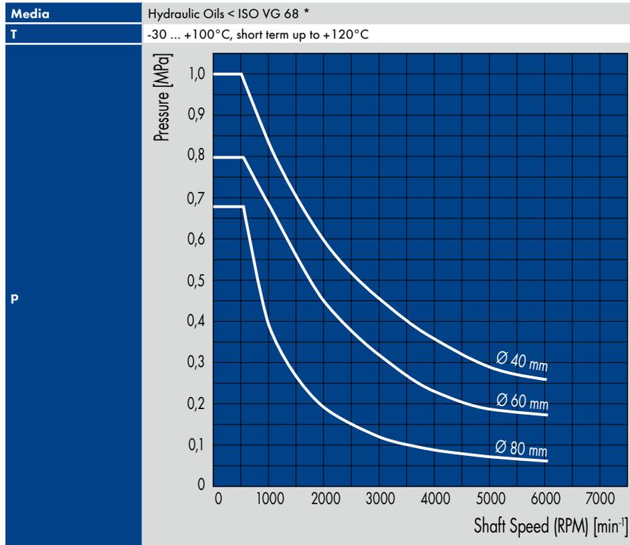
Permissible pressure in the unit for Simmerrings (type PPS)
